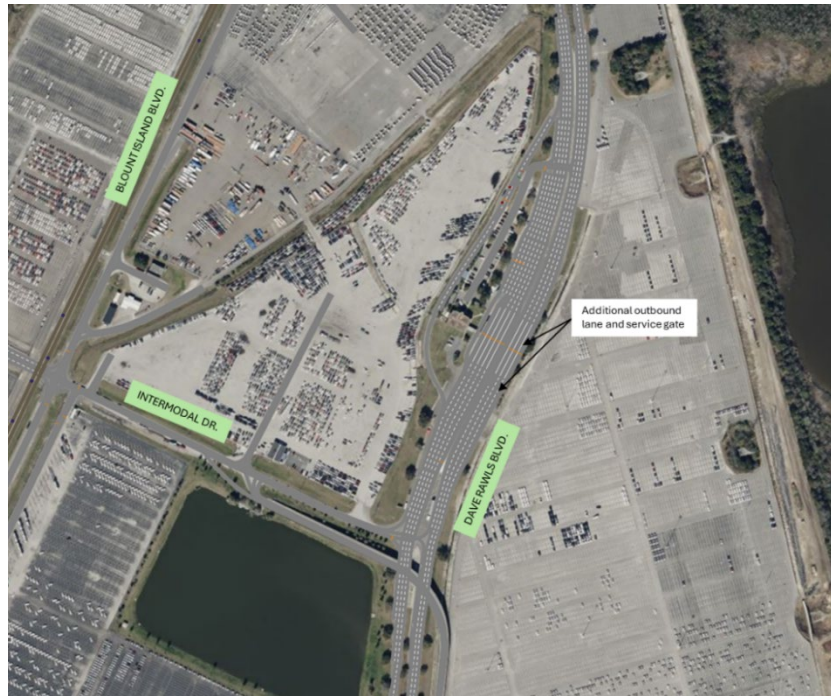
Figure 6-3 Additional outbound lane and service gate.
