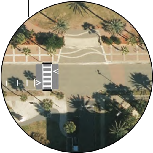
Add raised crosswalk
