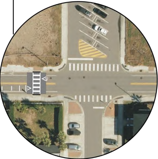
Add raised crosswalk
