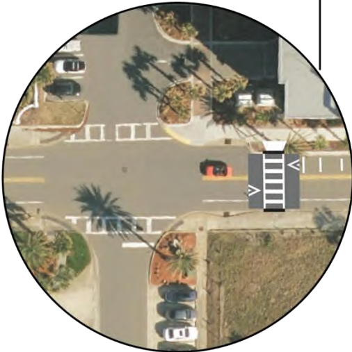
Add raised crosswalk
