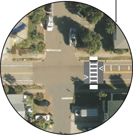
Add raised crosswalk
