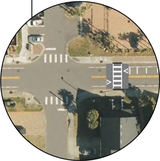
Add raised crosswalk
